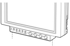
**4** Use the two screws to secure the main controls to the right panel.
